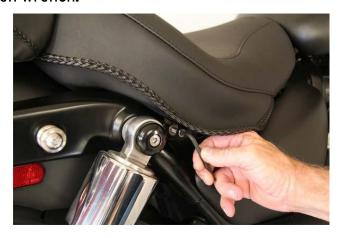
5. Align the solo's side brackets with the mounts on either side and install the stock 6mm bolts. Tighten both finger-tight, then tighten securely with a 5mm Allen wrench.
