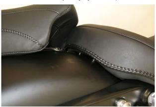
4. Install the stock 6mm rear screw through the rear seat bracket and into the fender. Tighten securely with a 5mm Allen wrench.
