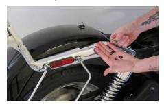
4. Remove the fender bracket (including nut, bolts and washers) from the fender using a 3mm Allen wrench and an 8mm wrench. Insert the black retaining clips into the two outermost holes in the fender.
